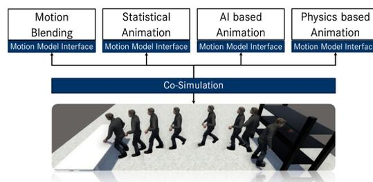
**Figure 1:** Principle of the novel approach, which couples heterogeneous character animation approaches by a standardized interface.
